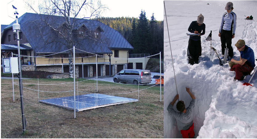
FIGURE 4.2 Climate station with snow scales in Modrava, Czech Republic (left), and snow pit close to the Furka Pass, Switzerland (right). Photograph: M. Jenicek.
